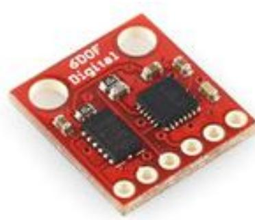
Figura 40 - IMU Digital Combo Board [49]
