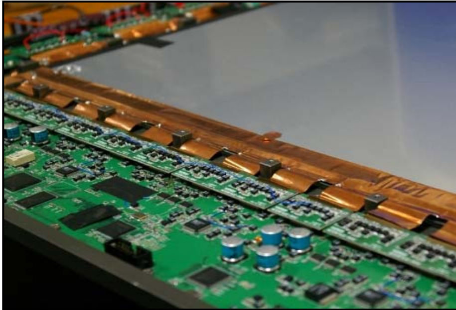
Figura 1.1 Samsung FXPD (flat-panel x ray detector) [17]
