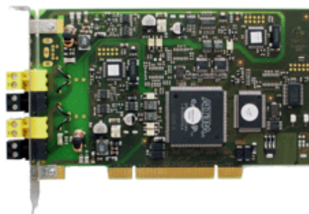
Figura 5-5: Placa PCI Board com 2 AS-i Master [21].
